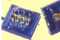
This tiny ZEN 360 direct plug decoder forms part of DCC Concepts' range of 8-pin DCC motor control decoders, designed to suit models where available space is at a premium.
